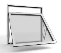
With the top swing ironmongery, the window sash can be pushed out and turned around 170° outside the frame, so the outside of the glass can be cleaned from the inside.
