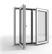
Frame with build-in "easy-clean hinge". windows has the advantage, that window cleaning may be done from inside. Hinges are hidden in the groove and has built-in adjustable friction. With the side mounted fitting, the frame may be opened 90° producing an opening of around 10 cm at the back edge of the frame - enough to reach out and clean the outer face
